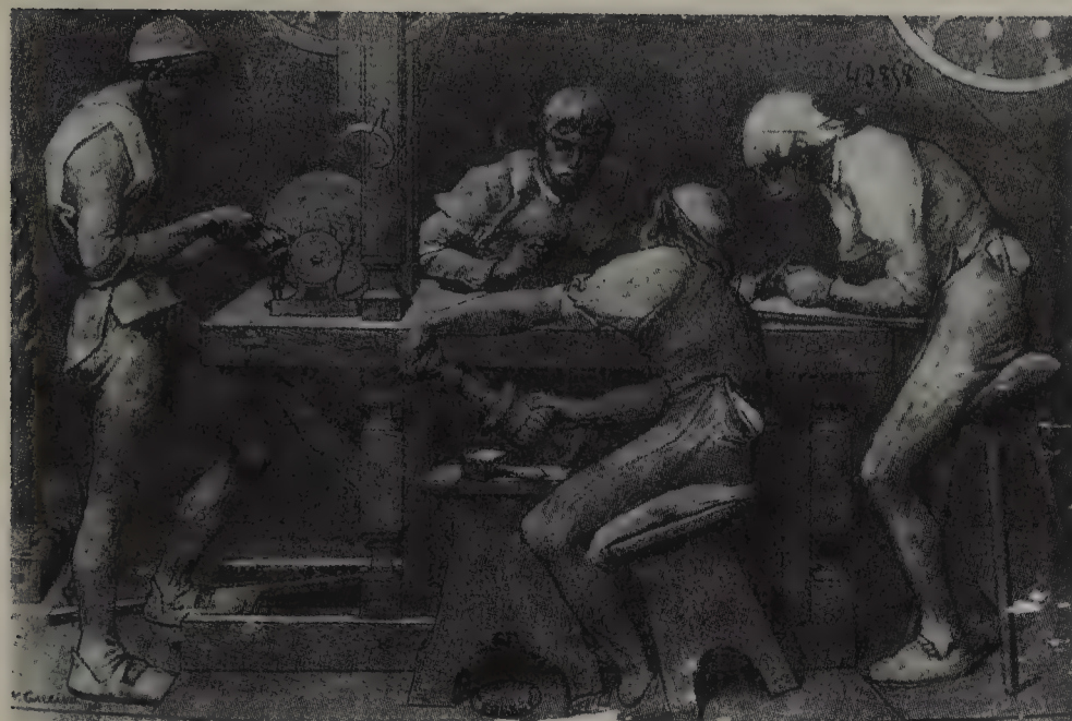
A wood turners' shop. This drawing dates from the late eighteenth century, toward the time when Bédé was born. Note the treadle-powered lathe at left. Bibliothèque Forney, Paris.
